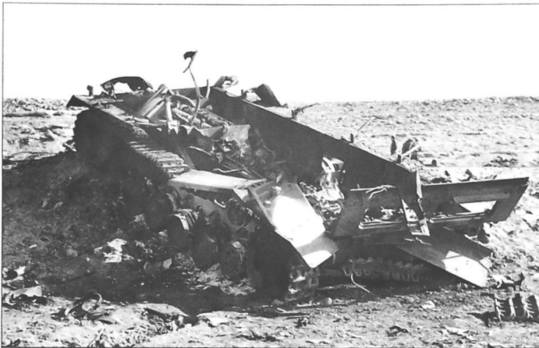
A photograph showing a Pz Kpfw III immediately after it received a direct round from a British tank. The vehicle has ignited and been literally blown to pieces. It is more than likely that tank shells that are stored inside the vehicle have caused the explosion.
