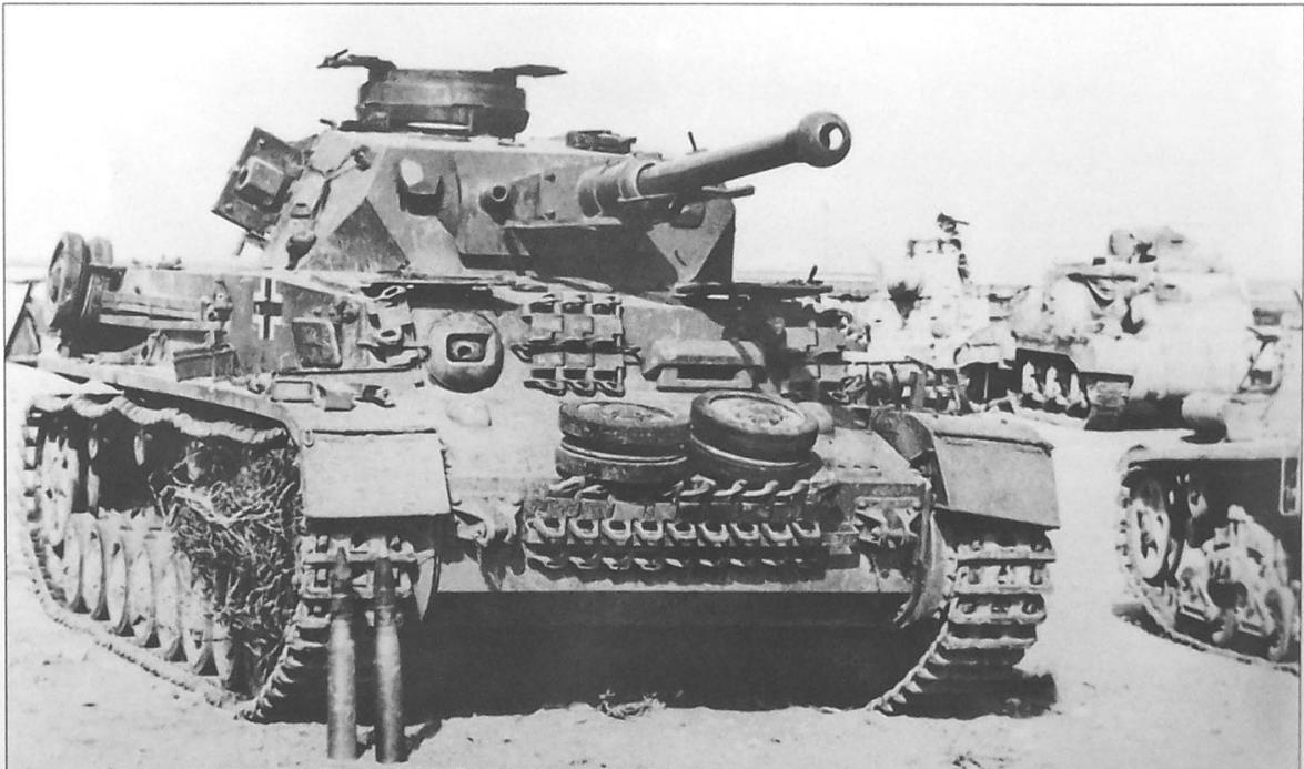
A photograph of a captured Pz.Kpfw.IV Ausf.F2 armed with a 7.5cm L/43 gun. The vehicle still retains its original color scheme of dark gray. Track links can clearly be seen attached to the tank's frontal hull for additional armored protection.
