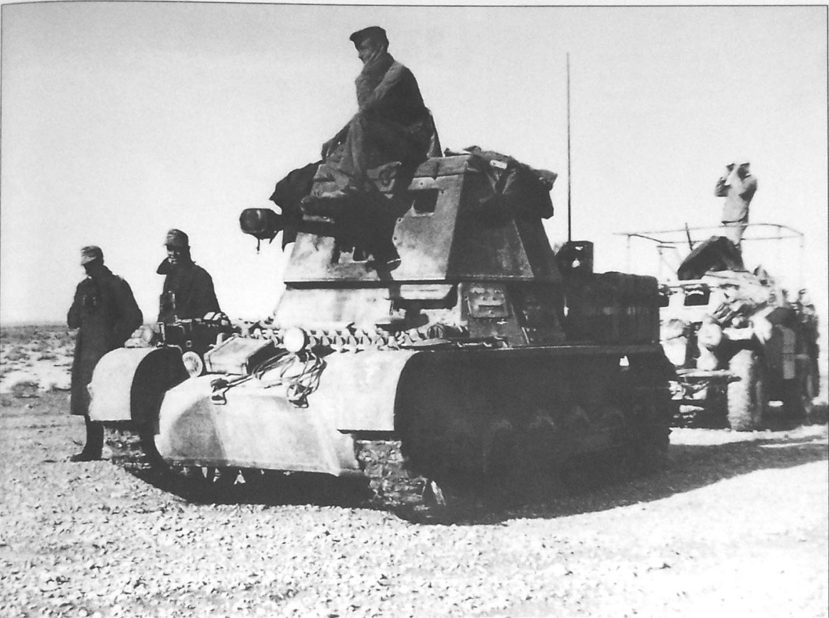
A Panzerjäger I attached to the 21. Panzer-Division is leading a column of vehicles out into the desert. This armored vehicle built on the chassis of a Pz Kpfw.I is painted in overall dark gray. The vehicle immediately behind it is an Sd.Kfz.223 being used primarily as an armored communication vehicle.
