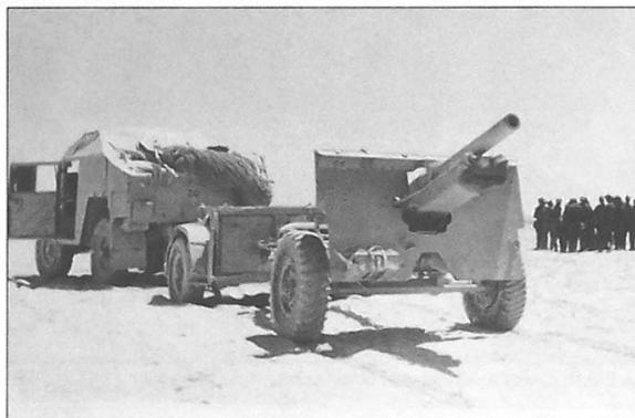
A captured British Morris C8 4x4 'Quad' field artillery tractor used for towing field guns and ammunition limbers. This particular Morris is towing a British 25-pounder, which was more than capable of knocking out Pz.Kpfw.I, IIs and even Pz.Kpfw.IIIs. A number of these guns and armored vehicles were used by the DAK against their former owners.
