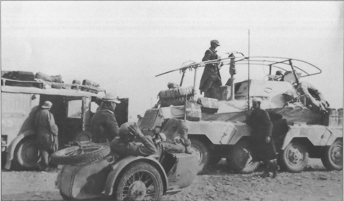
A dispatch motorcycle rider with combination halts next to an eight-wheeled Sd.Kfz.263 heavy armored car and Kfz.17 telephone exchange vehicle somewhere in the Western Desert in early 1942. As with all the vehicles issued to the DAK motorcycles too were also given a camouflage scheme of dark yellow and displaying the DAK Afrika palm symbol.
