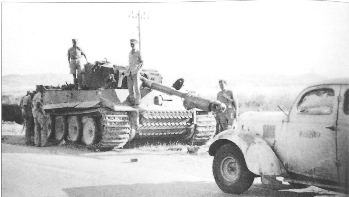
British troops examine a knocked-out Pz.Kpfw.VI Tiger I Ausf.E from sPz.Abt.504. This early Tiger I has its powerful 8.8cm gun barrel in a lowered position. The Tiger is painted in overall dark sand with a very light camouflage pattern of green patches.
