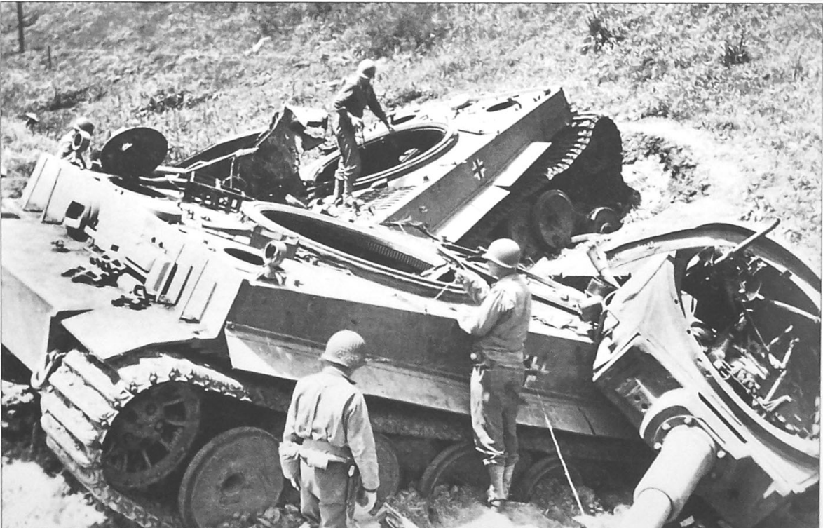
American troops survey the extensive damage wrought to two Pz Kpfw VI Tiger I tanks. Both of the vehicles have had their turrets blown off their mountings and lie next to the disabled tanks. It is more than likely that both of these Tiger's had run out of fuel and that the crews purposely destroyed them to avoid them falling into enemy hands intact.
