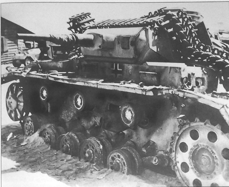
A badly damaged Pz.Kpfw.III Ausf.G without track links around its road wheels. One of its track links can be seen laid out across the hull. This vehicle is more than likely awaiting cannibalization for vital spare parts.
