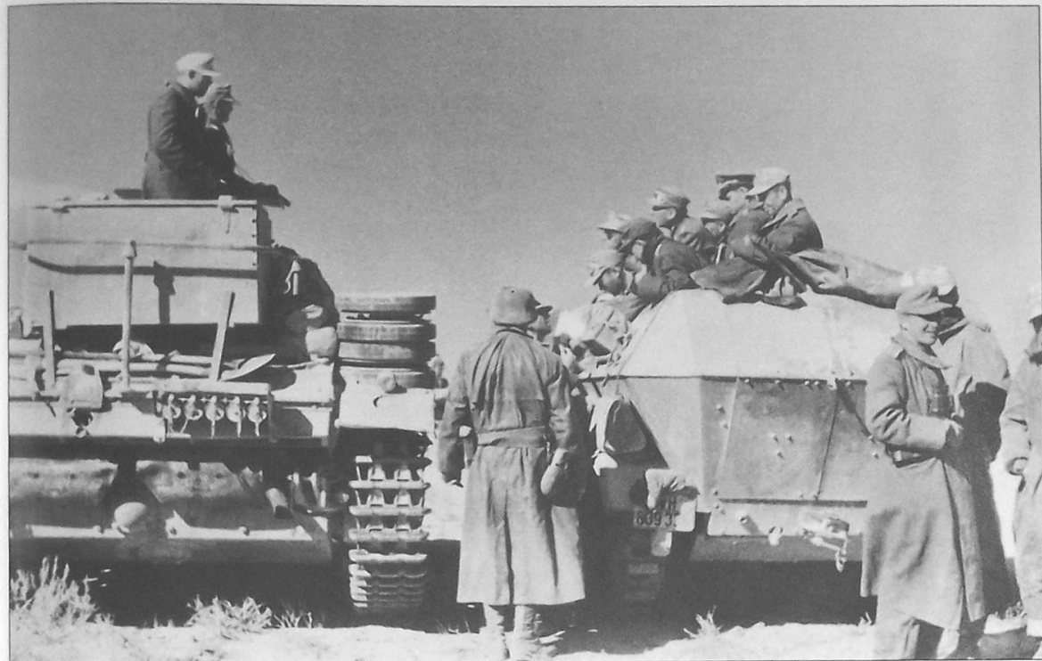
Success in the desert has now been restored. These troops from Pz.Rgt.5 have come to a halt in the Libyan Desert. On the right is a Sd.Kfz.251 half-track and on the left stands a well-laden Pz.Bef.Wg III Ausf.H, which is carrying a large stowage bin on the engine deck. Inside the box is the equipment needed to sustain the crew out in the harsh desert.
