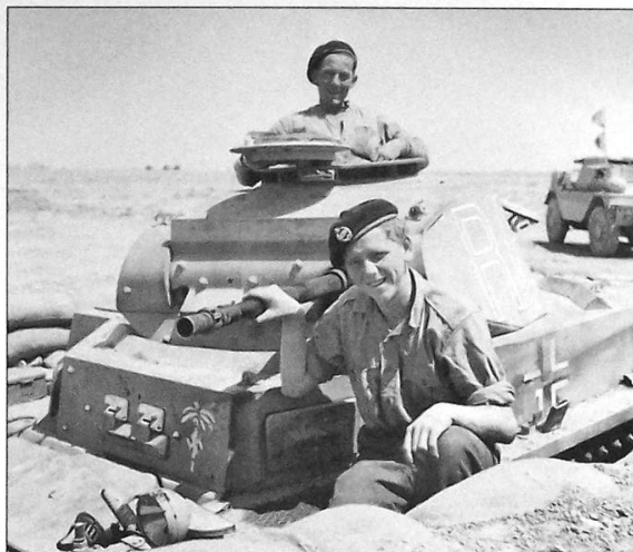
A Pz Kpfw.II Ausf A-C with a white outline tactical number 'RA' indicating it was assigned to the 'Regimental Arzt' or Medical Officer. The tank is in a fixed defensive position with sandbags and earth protecting the thin hull armored plating and road wheels. The tank is armed with a 2cm KwK 30 L/55 gun and was particularly effective in a defensive role, especially against lightly armed opponents.
