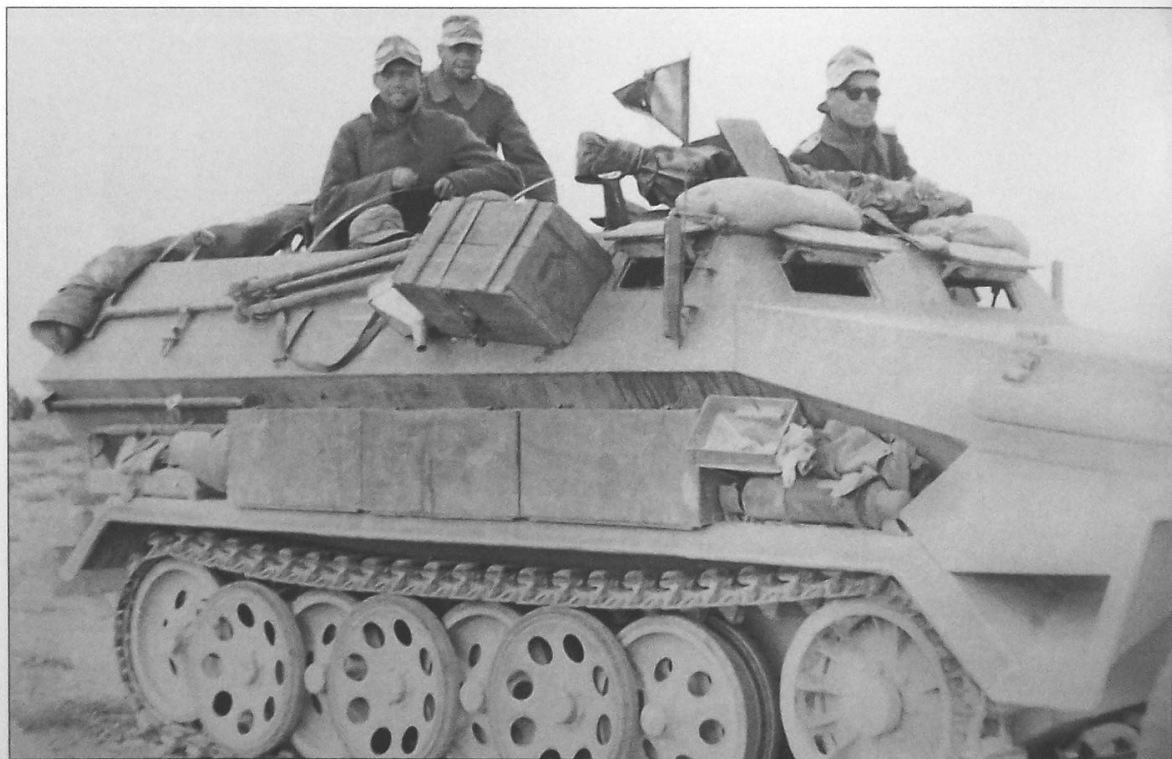
A Sd.Kfz. 251 Ausf. B command half-track has halted in the desert. Of interest is the MG-34 machine gun mounted on top of the vehicle, which has been wrapped in some canvas material in order to protect it against the desert sand. The half-track carries a hood and, like most DAK vehicles, is more than likely carrying the white transverse air recognition stripe. The half-track is painted in overall dark yellow and carries the divisional command pennant to denote the presence of an officer.
