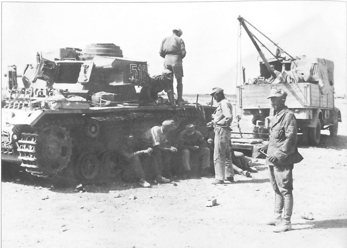
The majority of panzers in North Africa were lost in groups due to surprise fire from well-concealed batteries of enemy anti-tank guns. A DAK maintenance company, however, has salvaged this Pz.Kpfw.III Ausf.J, from complete loss. Much of the panzers armored success in the desert was owed to their well-equipped maintenance companies, which kept the vehicles in fighting condition. It appears that this particular Pz.Kpfw.III has experienced engine problems of some kind.
