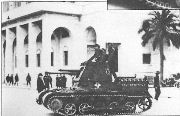
A Panzerjäger I assault gun moving along a road in Tripoli in February 1941. This vehicle still retains its original camouflage scheme of overall dark gray. The tactical number '13' is painted in white on the side of the fixed turret. The small national cross is painted in black with a thick white outline on the vehicle's hull-side.
