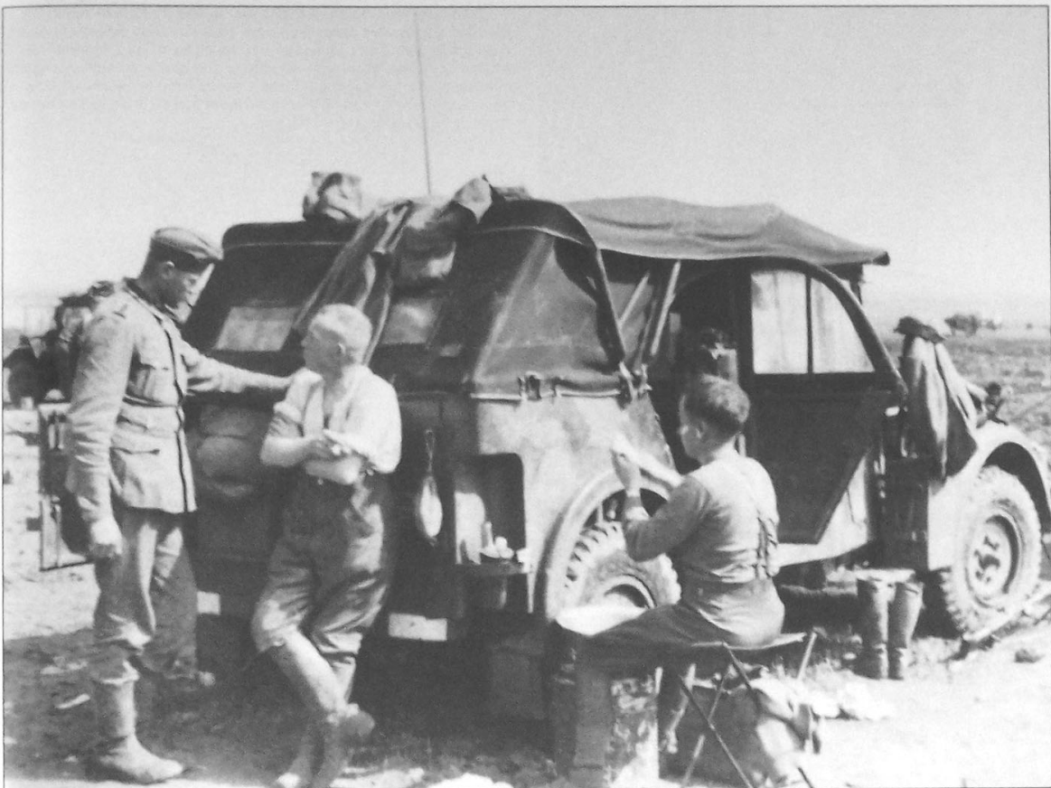
A Horch cross-country car with a crudely applied coat of dark yellow paint over the original dark gray color. The application of paint with a brush was widely adopted by DAK armored units, but the crude coating frequently left vehicles with patches of the original gray.
