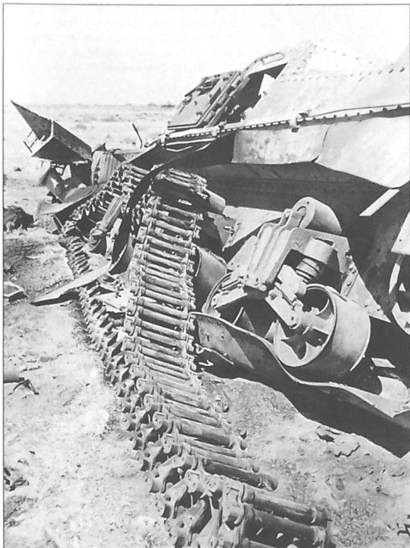
A Pz.Kpfw.IV Ausf.F2 has more than likely received an anti-tank shell round and as a consequence been knocked out of action. The vehicle has come to a halt in soft sandy terrain and its tracks can clearly be seen. The tank's 7.5cm long barrel is stuck in the elevated position. It is painted in overall dark yellow.
