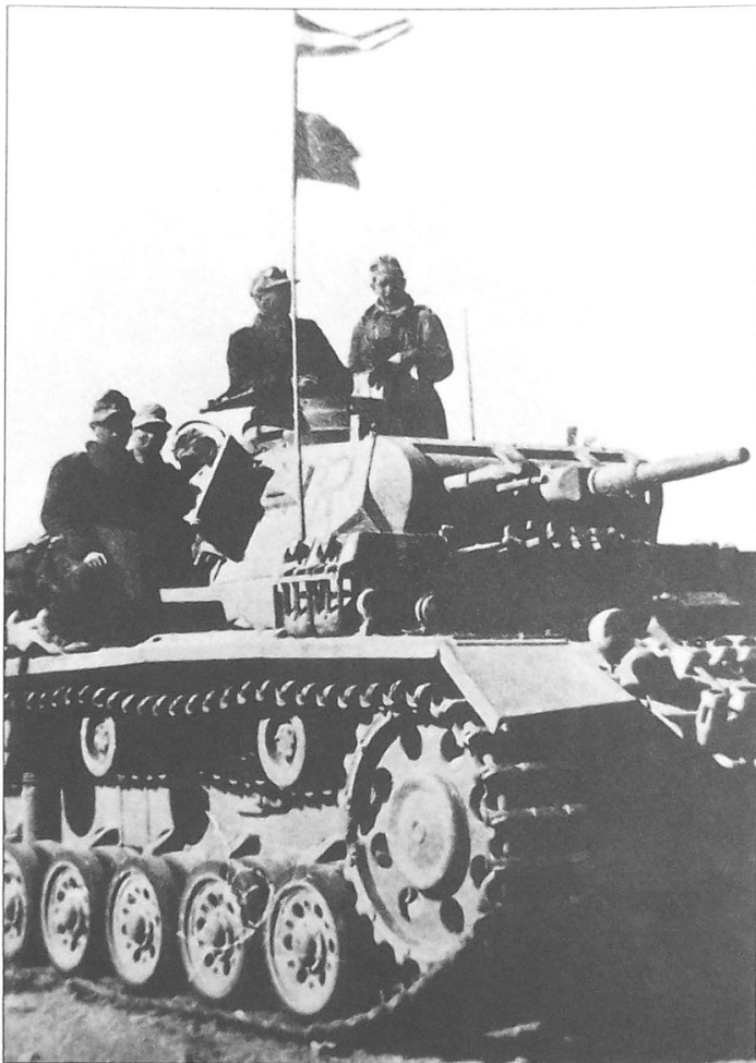
A Pz.Bef.Wg.III Ausf.H staff vehicle rolls through the desert. The tank is painted in overall dark yellow and carries the letter 'R' painted in red on the side of the turret. The letter 'R' signifies that it is a regimental staff vehicle. The tank is also displaying a command pennant for a panzer division in the DAK, which is painted in white, red and black.
