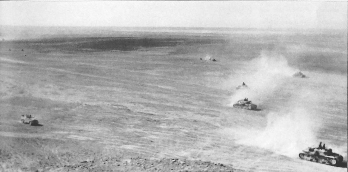
Several Italian Semovente da 75/18 assault guns advance across the open desert. This vehicle mounted a 75mm gun on a modified M13-40 or M14-41 hull.
