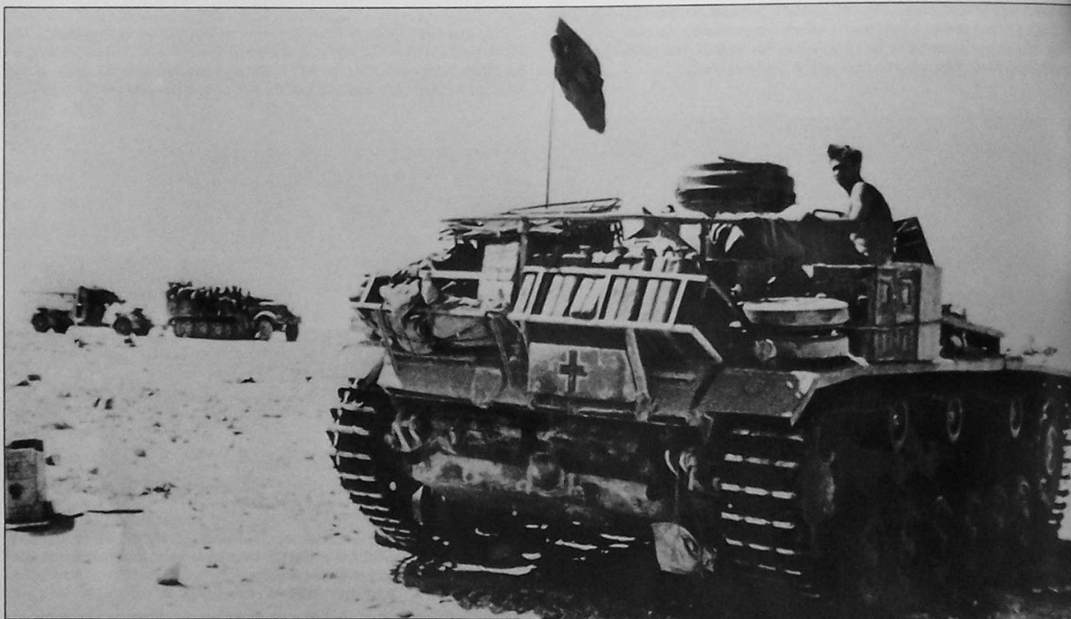
A very well laden Pz.Bef.Wg.III Ausf.H somewhere in the desert. Note the jerry cans and ammunition boxes and the specially built rack for containing all the supplies. In the background is a half-track with a full complement of crew towing an 8.8cm FlaK 18.
