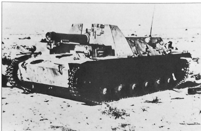
A 15cm sIG33 auf Pz.II has run out of fuel and been abandoned by its crew. The gun of this vehicle is mounted on the chassis of a Pz.Kpfw.II and there are six wheel bogie instead of the normal five. This vehicle was primarily used for close infantry support. It is painted in overall dark yellow and has a tactical number '404' painted in light yellow on the side of the hull.
